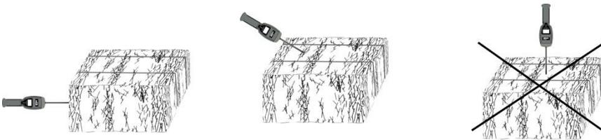
Do not push the probe all the way to the soft core of a round bale. Do not push to the flat end of a round bale.
