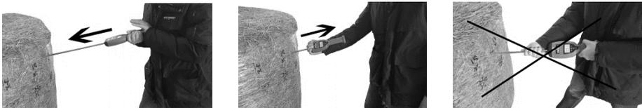
When measuring a bale with thick wrapping, puncture the wrapping with the probe tip before measurement to make sure the force required for making a hole in the wrapping will not affect density measurement.
